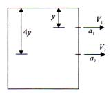
Volume of water flowing out per second from both the holes are equal.
